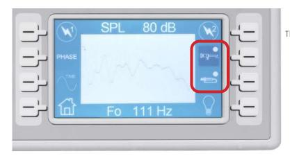
The device can be configured to be used with rigid or flexible endoscopes of different diameters. The microprocessor controls the work cycle of the LED flash, achieving images which are better balanced between light performance and image definition.
